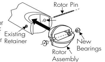
4. Tap the second retainer (rotor pin clearance hole inwards) into the hole while lining up the rotor pin with the center of the retainer hole. This completes the rotor replacement procedure.
