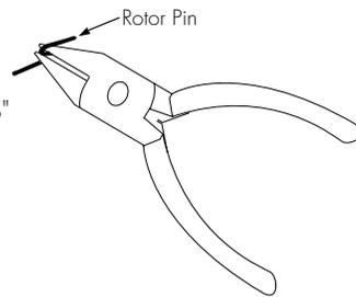
2. Remove retainer from each side by gently tapping it inwards using a punch. Install a new retainer with its rotor pin clearance hole inward. Only install one retainer at this time.
