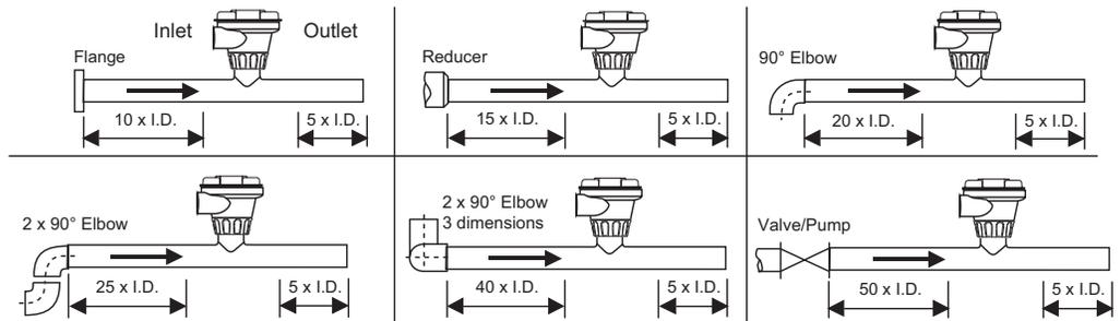
These configurations guarantee that the 2551 sensor will not be exposed to air bubbles when the system is in operation. These installations are recommended only if the system is designed to keep the 2551 sensor wet at all times.
