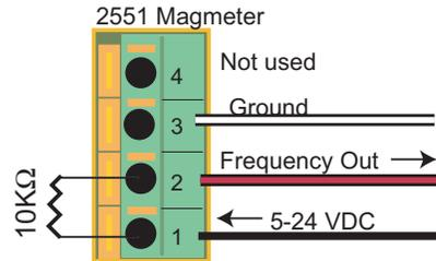
Install a pull-up resistor when connecting the 2551 Magmeter to other manufacturer's flowmeters.
