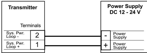
Connection to a PLC with built-in power supply
