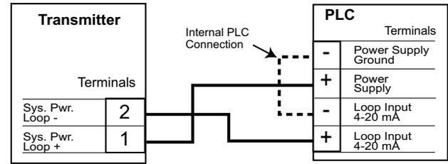
Connection to a PLC/Recorder, separate supply
