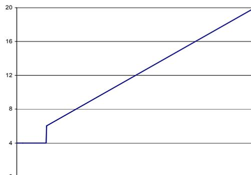
$$\text{Current Output (mA)} = \left( \frac{\text{Fluid Velocity in Pipe}}{\text{max Sensor Velocity}} \times 16 \text{ mA} \right) + 4 \text{ mA}$$
